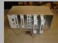
Fig.4 NI Signal Conditioner SCXI-1001
