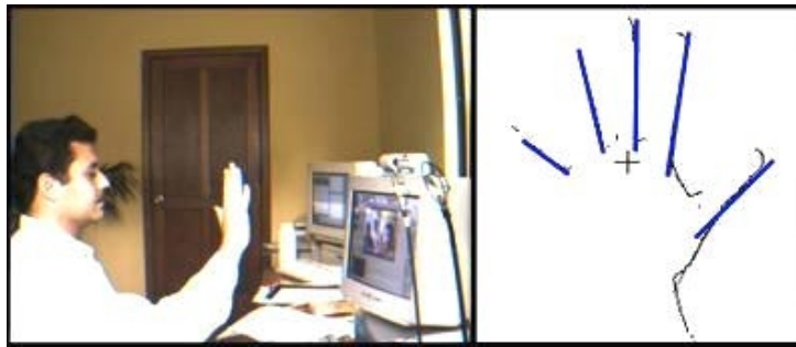
Fig. 4. Hand detector. This images show the way to establish the communication with the computer and the cursor defined by the fingers.
