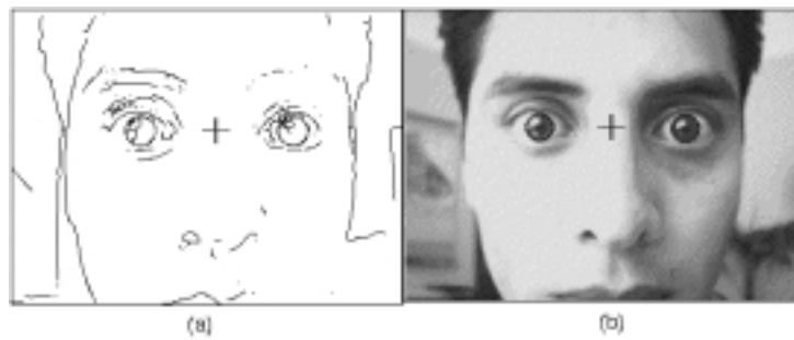
Fig. 3. Iris detector. (a) Edges on the image. (b) The mark represents the visual cursor which is defined by the position of the eyes.
